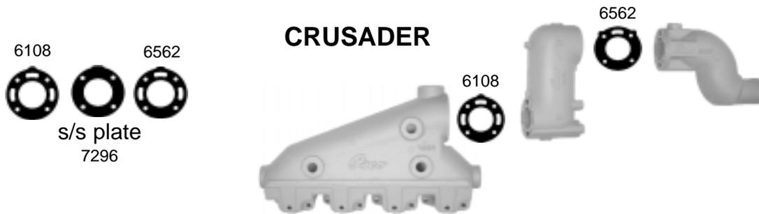
The round Crusader gaskets have tabs that stick up above the parts for easy identification. The “one hole” gasket has 2 tabs and is always used at the elbow. The “three hole” gasket has only 1 tab and is always used at the bottom of the risers to allow maximum water flow to fill the manifold and riser.
